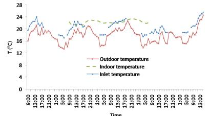
Figure 7a. Measured outdoor, indoor and inlet temperature, summer case.
