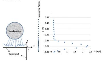
Figure 4. Profile of x velocity component in y direction, winter case.
