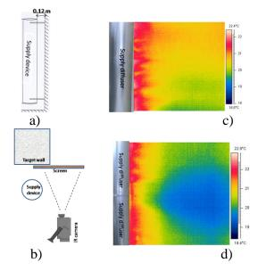
Figure 3. IR image visualization - supply air temperature about 22 °C, air-flow rate 0.25  $m^3/s$ , winter case a) side view b) top view set up c) one supply device d) two supply devices.
