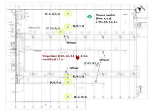
Figure 2. Geometry and position of the measuring points. temperature and humidity every 15 minutes during the measuring date, which was calibrated at the manufacturer.
