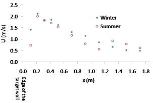
Figure 6. Decay of x velocity component in x direction at height 0.8 m from the floor.
