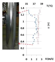
Figure 5. Profile of x velocity component and air temperature in z direction, winter case.
