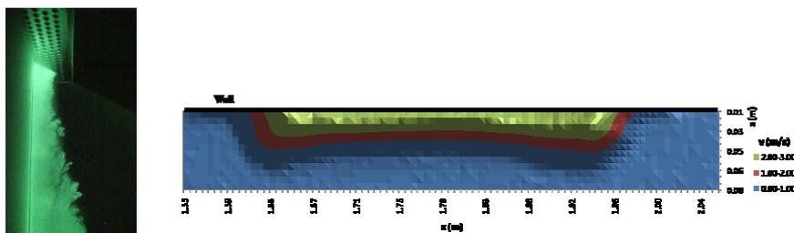
Figure 2. Flow pattern visualization by smoke (left) and the velocity profile 0.09 m below the diffuser used as inlet boundary conditions in the numerical simulation (right).
