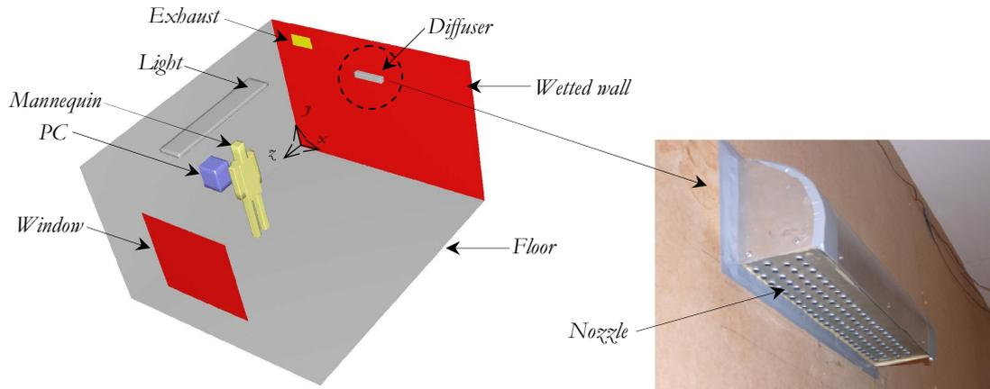
Figure 1. Test room layout (left) and the newly design supply diffuser (right).
